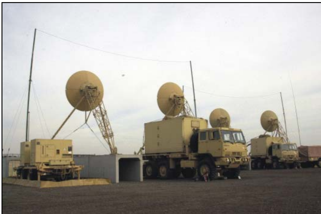
Figure D-10. AN/TRC-170(V)2 Heavy TROPO
