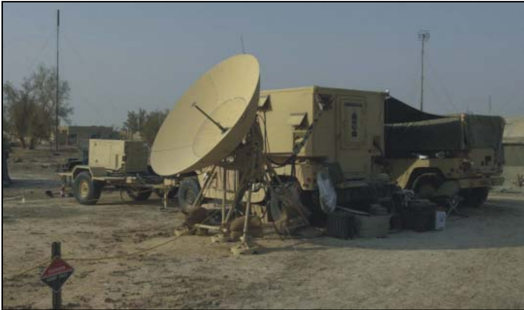
Figure D-2. AN/TSC-93 with 8-Foot Antenna
